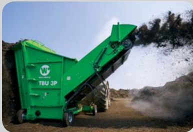
...► TBU in action: Restacking of trapezoidal heaps up to 3 meters with 0,5 km/h more
